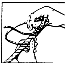
WRAP TWINE TIGHTLY AROUND ROPE STARTING 1/4 INCH FROM ROPE END.
