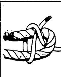
SHEET BEND FOR JOINING TWO ROPES TOGETHER OF DIFFERENT THICKNESS.
