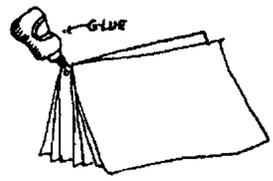
5. Put signatures together. Glue folded edges. Lay signatures on cover, as in next picture
