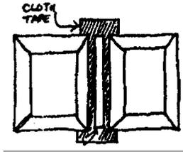
3. Place narrow strip of cardboard between front and back covers on a piece of cloth tape.
