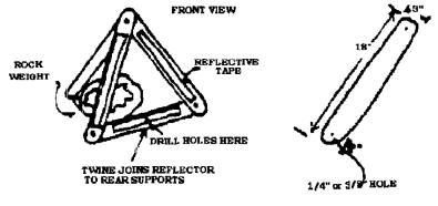
Cut paddles as shown. Cover one side of 3 paddles with reflective tape. Drill 1/4 or 3/8 inch holes as shown. In actual use, bolt or fasten the paddles together into a triangle shape as Illustrated. Fasten rear supports by tying with twine. Place the warning marker about 100' behind the disabled car parked on the shoulder of the road. Reflective tape faces oncoming traffic. Weigh down the bottom rear support with a large rock or something similar.
